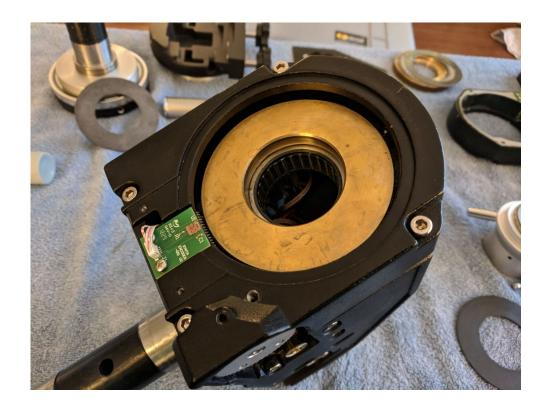
Loosely install the worm gear housing.
