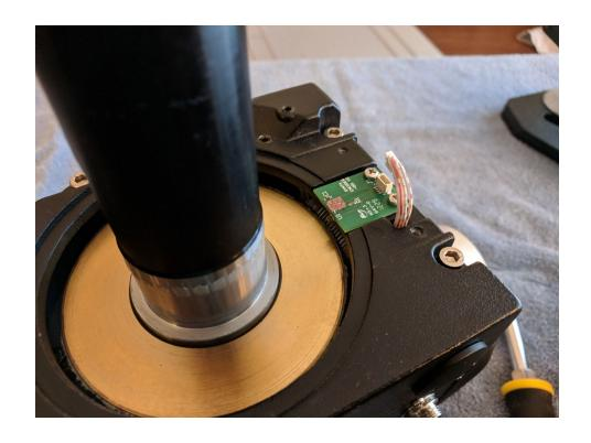
Remove the encoder wire cover with a phillips screwdriver and set aside.
