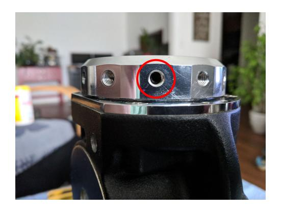
There are three set screws hidden under the RA tension clutch ring. Carefully rotate the clutch ring until you can see a set screw.
