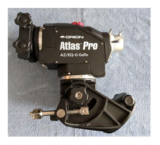
Install the mount head casting. Secure with the two pivot shaft pins and fully tighten them.
