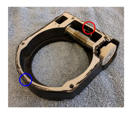
The worm engagement adjustment is critical. It is a balance between low backlash, and gear binding. The goal is to adjust for minimum backlash without introducing binding in the worm gears.
