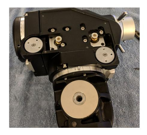
With the drive motors loose and the drive belts removed, we can now disassemble the RA axis.
