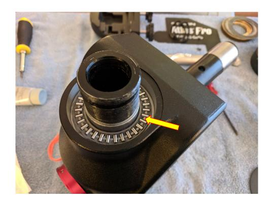
Install the small thrust bearing on the end of the DEC shaft. Ensure that the assembly order is washer, roller cage, washer. Work grease into the roller cage with your fingers.
