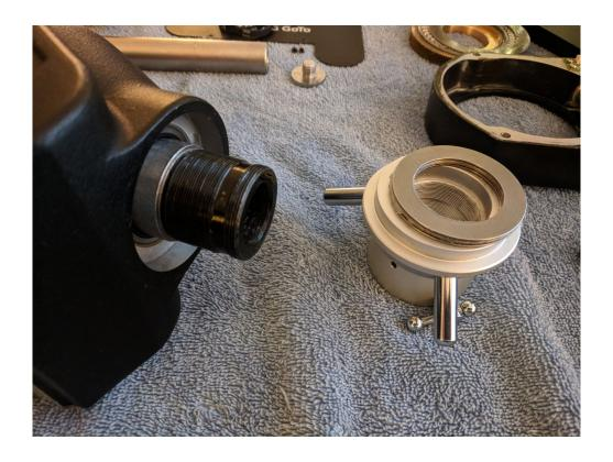
Remove the thrust bearing and set aside. Be careful to ensure that all three bearing pieces remain together.
