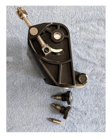
Set aside the two pivot pins and the altitude adjustment pin.
