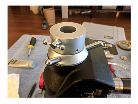
Install the DEC tension clutch ring, threading it tight until the DEC clutch locks up.
