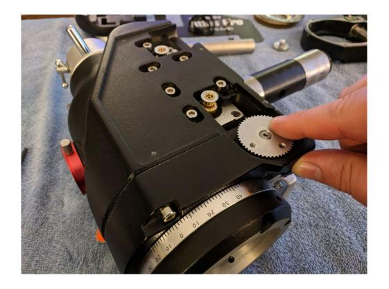
Both binding and backlash can be felt by spinning the DEC worm drive gear with your finger.
