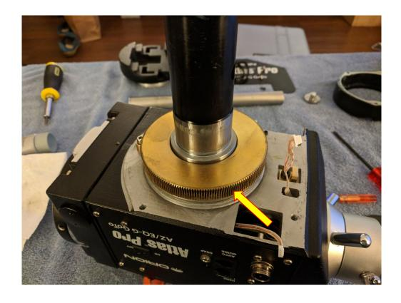
Install the RA worm ring on top of the thrust bearing. Use your finger to spread a small amount of grease into the worm ring teeth. Put the grease all the way around the worm ring.
