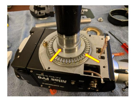
Re-assemble the large RA thrust bearing. Ensure that the assembly order is washer, roller cage, washer. Work grease into the roller cage with your fingers.
