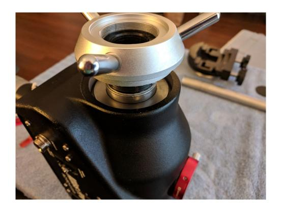
Unscrew the DEC tension clutch ring and set aside.
