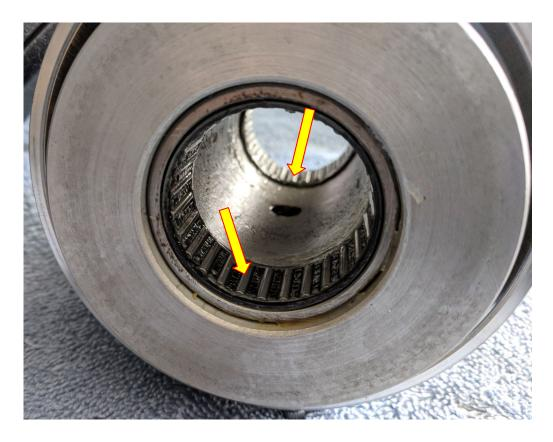
Grease both RA axis radial roller bearings. Work the grease into the bearings with your finger.
