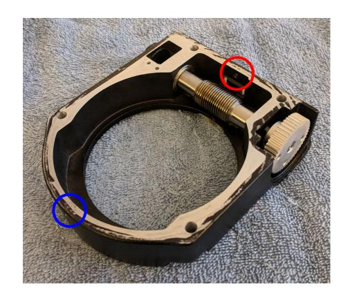
The set screw circled in blue (ring side) pulls the worm gear into the worm ring. This decreases the gear interface spacing. Lower spacing results in a smaller amount of backlash (good), but increases the chance of gear binding (bad).
