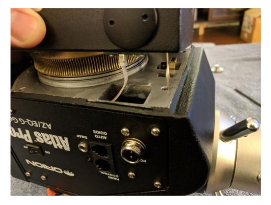
Just like on the DEC axis, loosely install the worm gear housing.
