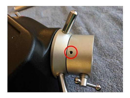
Remove the three set screws that secure the DEC end cap in place with a 2mm allen driver.
