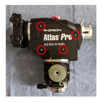
Remove the four phillips screws holding the motor cover in place.
