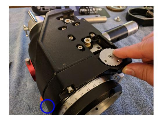
If you can rock the gear back and forth several degrees without any motion on the DEC shaft, you have excessive backlash and need to tighten the ring side set screw and loosen the worm side set screw
