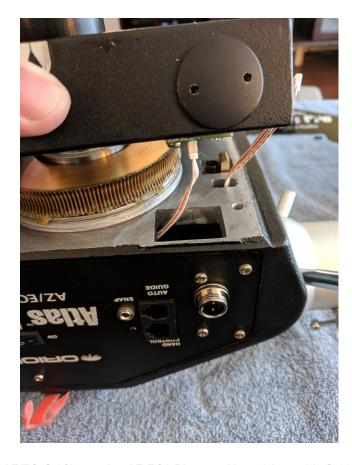
Carefully lift the worm cover, feeding the encoder sensor wire down through the hole it is routed through.
