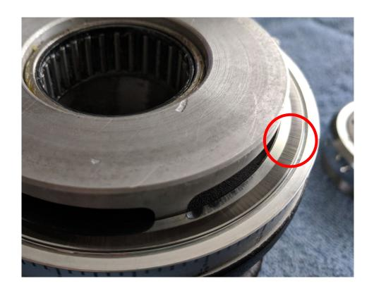
The RA encoder sensor ring is located on the underside of the RA casting. You can see the fine lines in this image that are picked up by the encoder sensor.
