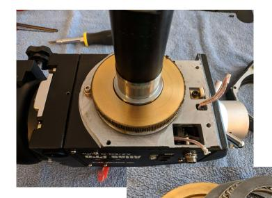
With the worm cover removed, you can remove the worm ring.
