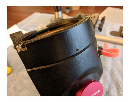
Like with the RA worm housing, remove the encoder sensor wiring cover and set aside.
