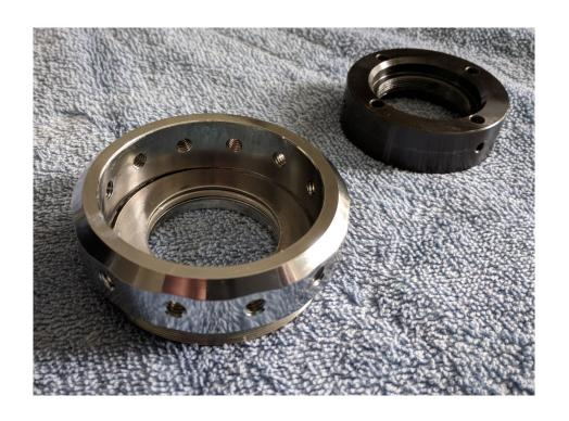
With the end retainer removed, the clutch tension ring can also easily be unthreaded and removed.
