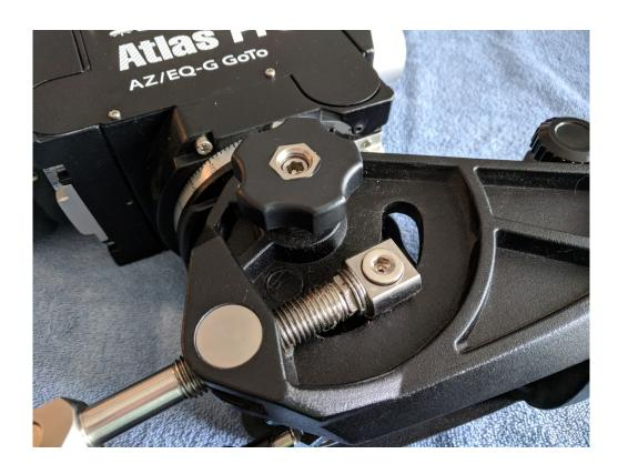
Loosen the two plastic knobs on each side of the altitude adjustment axis.
