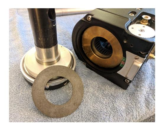
With the clutch tension ring and end cap removed, the DEC axis shaft can be carefully removed from the mount housing.
