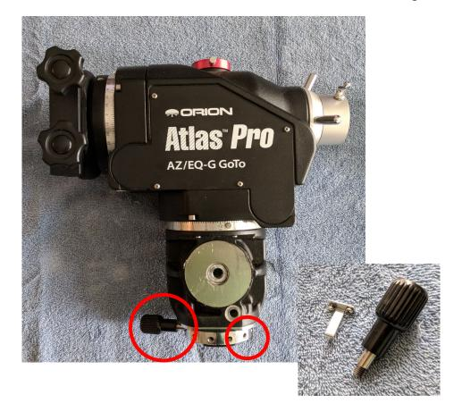
Remove the polar scope if installed.
